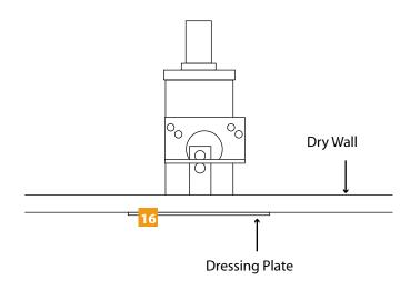
17 Replace and tighten two #6 screws on opposing sides of the 2" electrical box so that the spring tabs on the side of the 2" electrical box push out against the drywall and secure the box in place.
