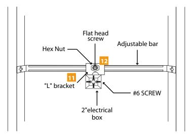
**16** After installing the drywall, place the dressing plate on the 2" electrical box. The dressing plate should cover the plaster or open spaces around the 2" electrical box.
