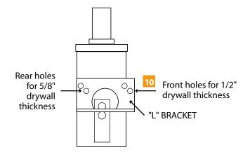
10 For 1/2" drywall thickness mount the "L" bracket on the 2" electrical box by using the two front holes. For 5/8" drywall thickness mount the "L" bracket to the 2" electrical box by using the two rear holes.
